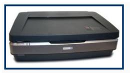
A highly sensitive flatbed scanner for most common nonfluorescent densitometric applications in the life sciences, especially electrophoresis evaluation. The scanner has a linearity above 3.4 OD, with 16-bit pixel depth, providing accurate quantitation and high sensitivity of very faint images without additional filters.
