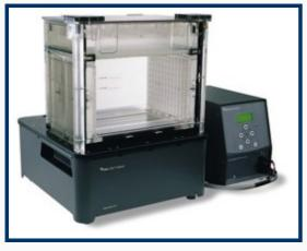
Ettan DALTtwelve System can run simultaneously up to 12 large-format gels in4 to 6h. The system streamlines performing second-dimension SDS-PAGE separations, increasing productivity while delivering high throughput, resolution, and reproducibility. When used in combination with 24 cm Immobiline<sup>™</sup> DryStrip gels, Ettan DALTtwelve maximizes the number of discrete, quantifiable protein spots obtainable per large-format gel.
