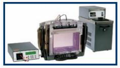
Ettan<sup>™</sup> DALTsix Electrophoresis Unit runs up to six large format (26×20cm) second-dimension polyacrylamide gels in just 4-5h. The gels accept first dimension 18- or 24-cm Immobiline DryStrip gels (IPG strips) from both Ettan IPGphor<sup>™</sup> and Multiphor<sup>™</sup> II isoelectric focusing systems. The system components include Ettan DALTsix Electrophoresis Unit, Gel Caster and Gradient Maker, an EPS 601 Power Supply, and MultiTemp<sup>™</sup> III Thermostatic
